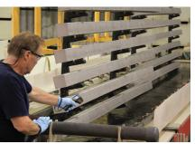
MetCon technician checks the electrochemical bath temperature as material is loaded into a tank. The MetCon process environment requires none of the haz-mat precautions typically associated
