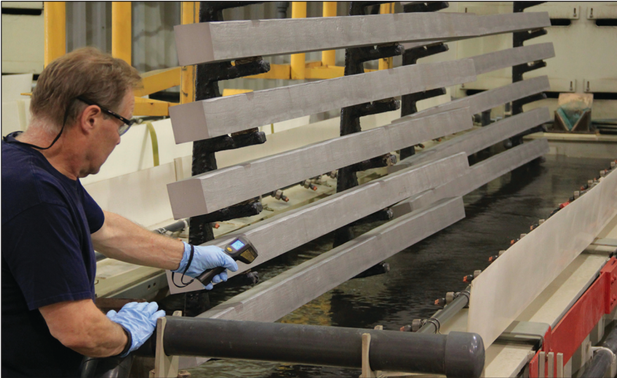
Technician checks electrochemical bath temperature as material is loaded into tank. The green MetCon process environment requires none of the extreme hazmat precautions typically associated with pickling.
