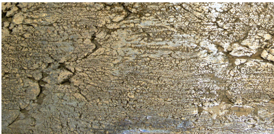
As forged incoming material displaying cracks and alpha case, requiring conditioning.
