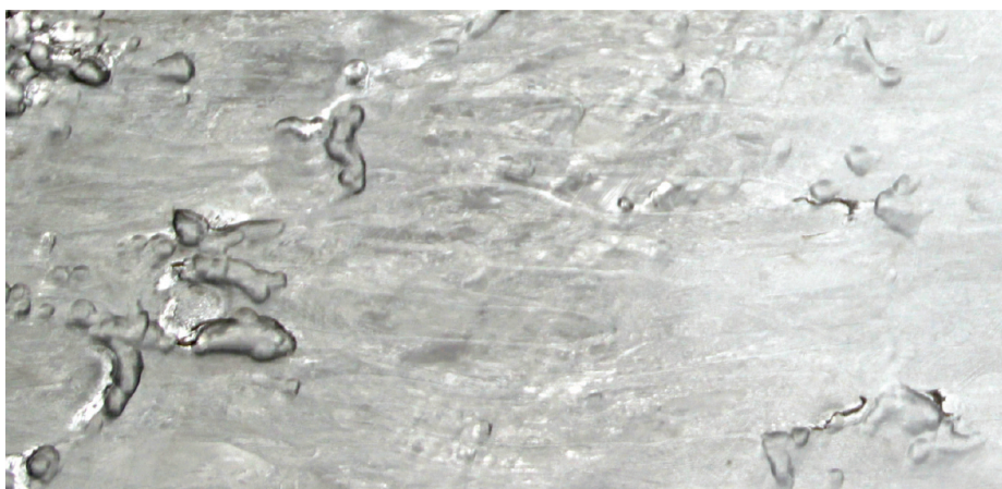
The same material fully conditioned by the MetCon process, ready for forging or rolling. Crack tips have been removed and more parent material is preserved than by traditional conditioning methods.
