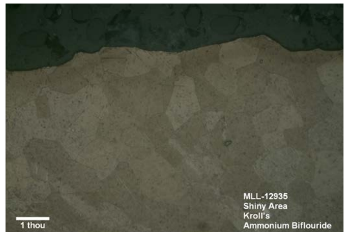
Figure 7. Metallographic Specimen Prepared in Shiny Area with No Indication of Alpha Case
