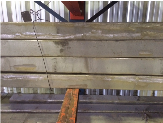
Figure 9. MetCon Processed 100 mm (4") Square Bars Showing Representative Spot Grinding
