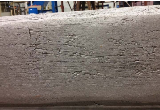
Figure 4. As-Forged and Blasted, 23 cm across the flats (9 inch) RCS Ti-6Al-4V Bloom Requiring Conditioning Prior to Subsequent Forging (Source: MetCon)
