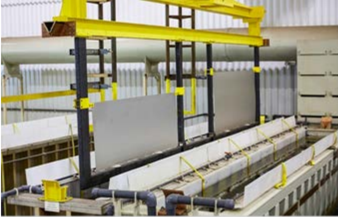
Figure 11. Sheet/Plate Rack Supporting up to One (1) 10 cm x 152 cm x 660 cm (4" x 60" x 260") or up to Two (2) 10 cm x 15 2cm x sum to 635 cm (4" x 60" x sum to 250") Sheets or Plates
