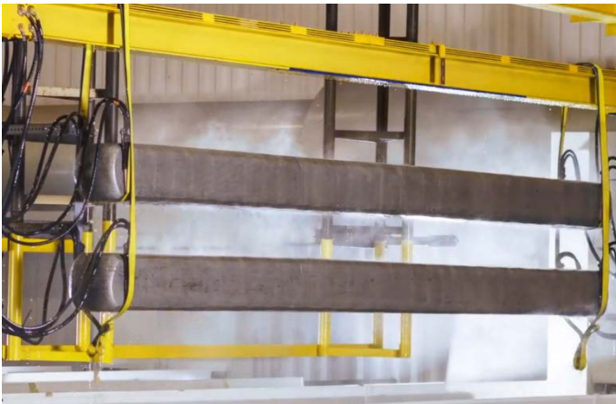
Figure 12. Lifting Straps Able to Accommodate Any Product Up To 81 cm x 167 cm x 66 0cm (32" x 66" x 260") and Less Than 8100kg (8 ton)
