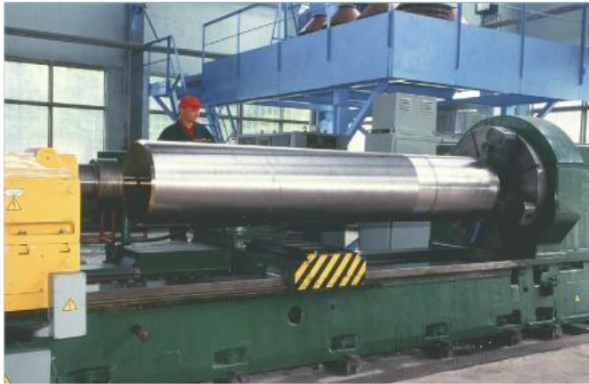
Figure 1. Lathe Turning Titanium Ingot (source: Antares)
