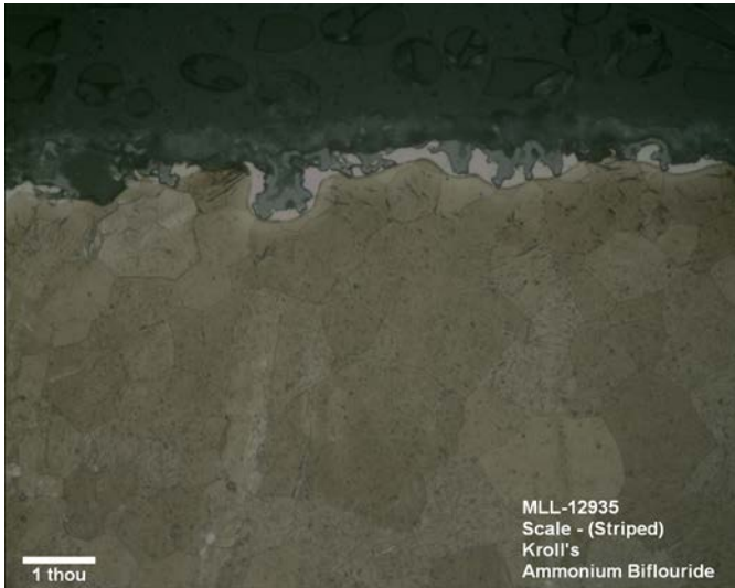
Figure 8. Metallographic Specimen Prepared in Area of Discontinuous Black Marker. Alpha Case Layer is Indicated.
